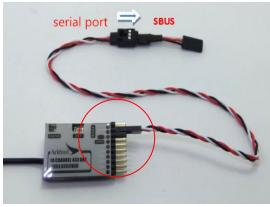
On the Arkbird OSD 1.0, the original 1-4 channel input ports which used to connect common receivers, automatically become output ports which will output the controlling value of channel 7-10 of the remote control.
