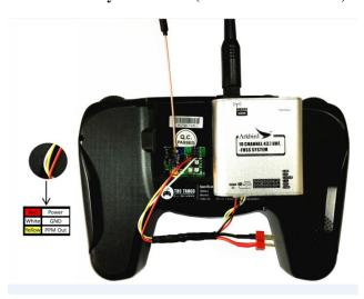
In PPM mode, Radio (Plug T not connected) will supply power for head tracker receiving module and 433 UHF transmitter. PPM signal from radio will be sent to receiving module of head tracker, which will imposes pitch and roll control values to PPM signal Channel 7 and Channel 8. The signal will be sent to 433 UHF.
