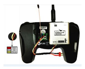
In PPM mode, Radio (Plug T not connected) will supply power for head tracker receiving module and 433 UHF transmitter. PPM signal from radio will be sent to receiving module of head tracker, which will imposes pitch and roll control values to PPM signal Channel 9 and Channel 10. The signal will be sent to 433 UHF.
