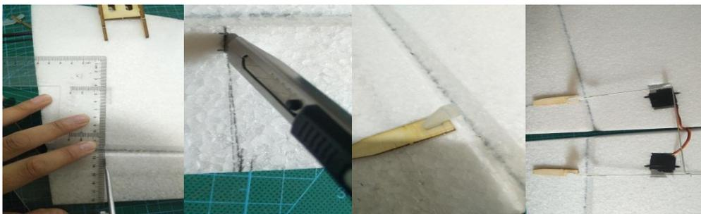
Assemble rudders: cut a notch of 5-8mm long and 6mm deep in the foam as above. Then stick glue around the notch and its inner part. Place the rudders in the right position as shown above. Remind keeping them in alignment with front edge of servo surface.
