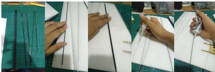
Pick out the carbon rods and carbon chips in the picture. The carbon chips are used to strengthen airfoil and carbon rods are used to strengthen plane control surface. Stick the carbon rods with glue 502 and stick the carbon chips with foam glue.
