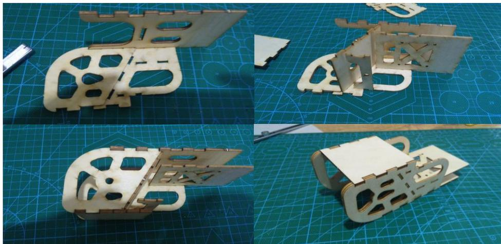
Next, assemble the main fuselage. Follow pictures shown above to stick these parts to the wooden nose. Ordinary foam glue is alright for this.
