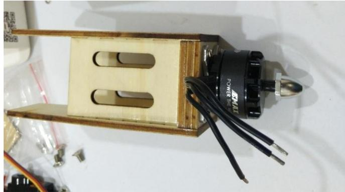
M3 sunk screws, motor mounting base, flat tail tapping screws and shim are packaged in the accessories bag. Please install them on motor mounting base. The finished assembly is as shown above. There are two set, one for each motor.
