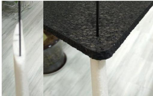
Assemble wing fence. Using toothpick or other tools to fix position. Then stick glue to it.
