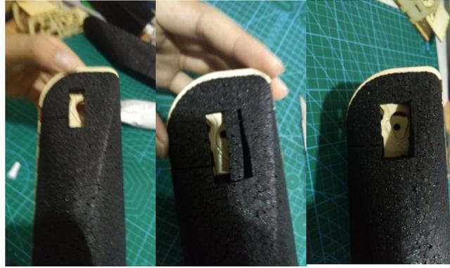
Attention. The wooden holes may not be in alignment because of size errors. Please carve a slot of 5-6mm long to suit the position of left servo.
