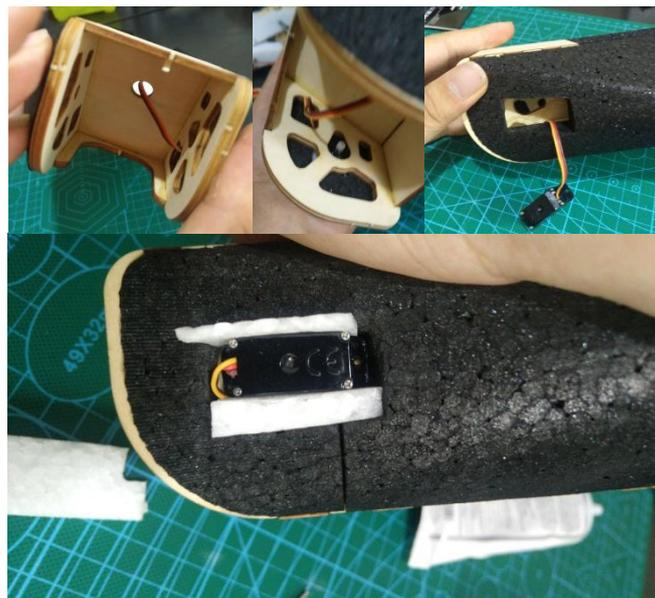
String the servo cables following the picture. Use wasted foam to prepare two chips to fix the position of servo. The size of chips depends on servo position and installation holes. Stick the chips with foam glue. Then cut off the excess parts.
