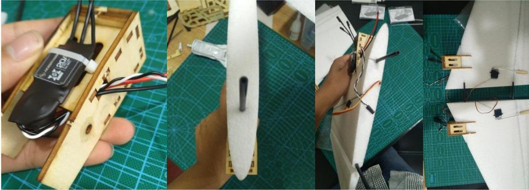
Meanwhile, install the ESC as shown above left picture. Locate 4 carbon rods of 5mm, 2 carbon rods are long and 2 carbon rods are short. Then assemble the ESC with motor base to the airfoil. The short carbon rods will go through the motor base as shown in the picture. But only the carbon rods are to be glued. The motor base should not be glued, it is the final step to fix motor base. The side assembled with ESC is belly of plane. The side assembled with servo is back of plane.
