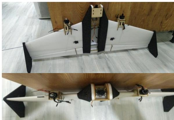
Put the autopilot beside a flat side of desk to make sure wing fences (undercarriage) are in right position.
