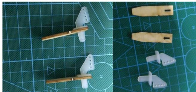
Preparing rudders: pick out rudder parts and stick them with glue 502 as shown in the pictures. Remind keeping the front edge in alignment.
