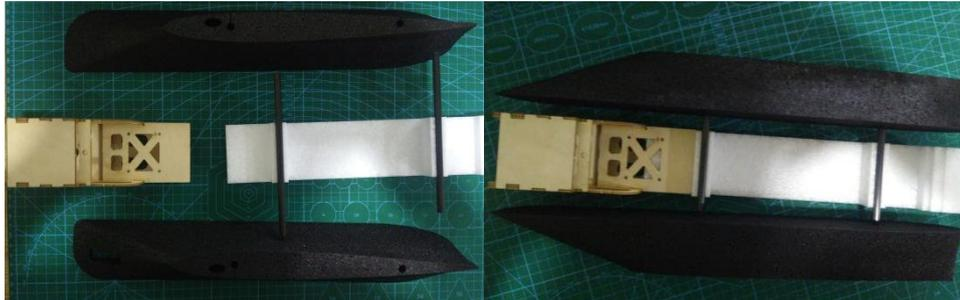
Assemble fuselage. Pick out the foam in the picture and pose the two carbon rods of 7mm as above. Then fix them by sticking glue to the foam and carbon rods.
