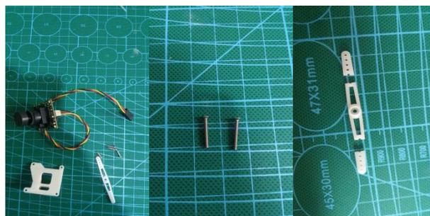
Pick out camera base. Using long rocking shaft and screws to install camera into camera base. The camera is compatible with Arkbird camera. The screws of M1.6\*14mm are included in the parts package.
