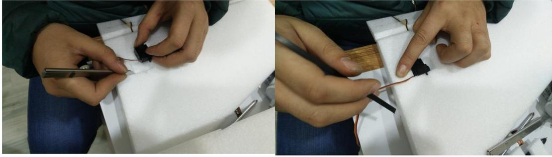
Assemble servo: cut a notch of 5mm deep in front of the servo installation slot. Then press servo cables into the notch. DON'T glue the servo at the moment.
