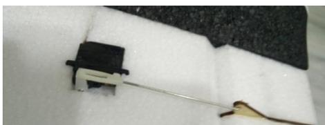
Assemble push rod and control horns as shown above. They are assembled into the elevons hole at the outermost side.
