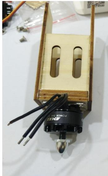
M3 sunk screws, motor mounting base, flat tail tapping screws and shim are packaged in the accessories bag. Please install them on motor mounting base. The finished assembly is as shown above. There are two set, one for each motor.
