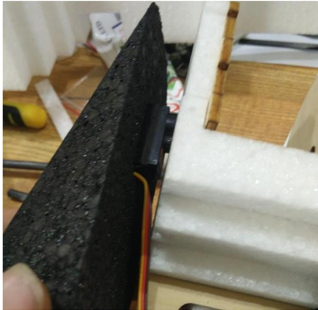
Then, we use the black wing shoulder to stick to the left side and assemble servo as shown above. Place the wires into the slot.
