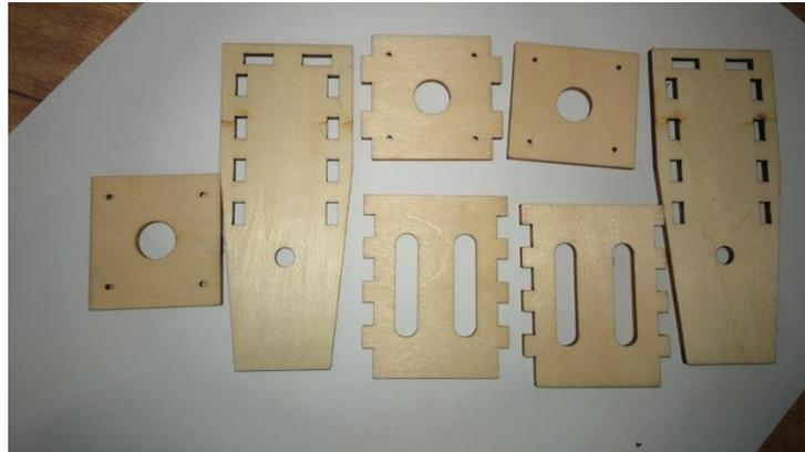
Picking out the parts to assemble motor mounting plate as shown above.
